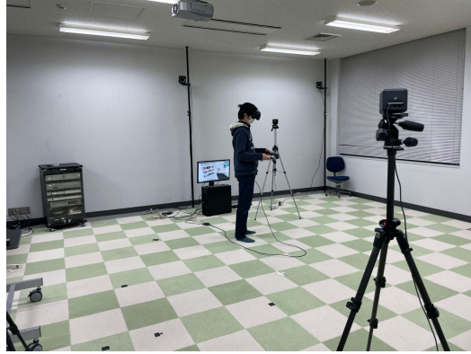
Fig. 4. Experiments were conducted in a room-scale VR environment of 6.8 x 6.4 meters using HTC VIVE.
